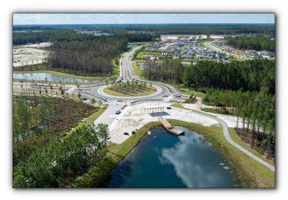
Our scope of work included layout staking for clearing limits, fencing. and construction, as well as establishing site control for GPS-guided machinery. We also conducted post-grading topographic surveys and provided as-built reviews and certifications. Through efficient pre-calculated layout process and daily field reporting, we ensured precise and timely support throughout the project's development.
